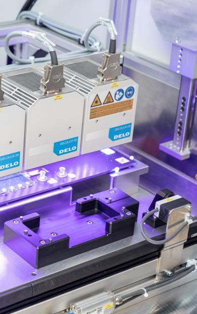
In downstream cells, for example, connecting parts can still be bonded to the front glass. After automated optical bonding is complete, a visual inspection is usually carried out by experienced machine operators, after which the displays are ready for further processing. Using these systems, PIA Automation reaches cycle times of around one minute.
