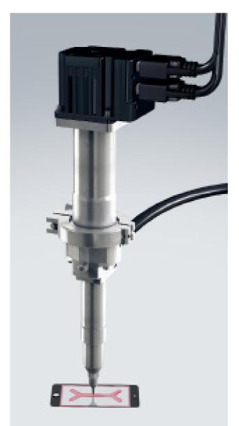
An important prerequisite for perfect bonding processes is that the bonding fill compound is applied to the respective components via metering systems in the desired quantity and viscosity.
